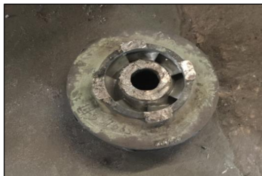
구축함 Cooling Water Pump Impeller
