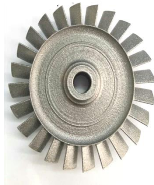
Inconel 718 rotor part ( \varnothing 125mm x 30mm) Printing time: 15h
