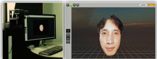
Figure 1. Face Capture using Depth Sensor
